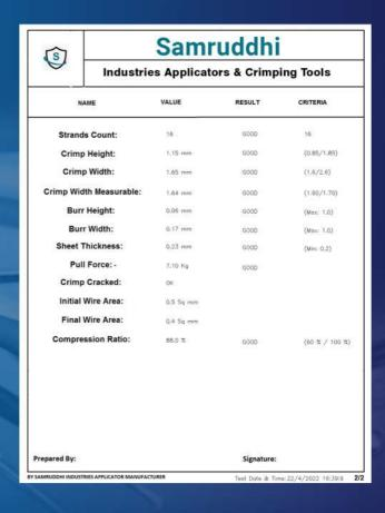
It is said that Applicators are the heart of the Crimping process, this is why quality maintenance is of critical importance. successful Crimping results from the correct relationship between wire, terminal, & crimping tool. once the terminal selection is made & Crimping criteria defined by the connection designer, the tooling characteristics are fully determined.
